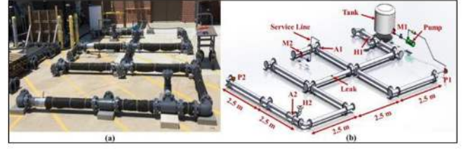
Fig. 2. Experimental Water Distribution Test Bed in a Branched Topology Configuration
